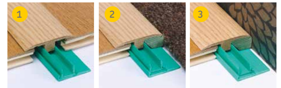
Expansion Profile to cover expansion gaps between two adjacent flooring products of the same height. Adaptor Profile for use when finishing between two adjoining floor coverings where the adjacent floor covering is of a lower height e.g. carpets or vinyl. Edge Profile to finish the flooring where a dressed edge is required eg. against a wall or window.
